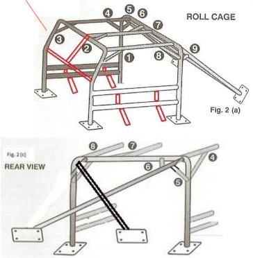
Corner gusset bars are included in the diagrams to be added as a means to add weight to the car if necessary.
